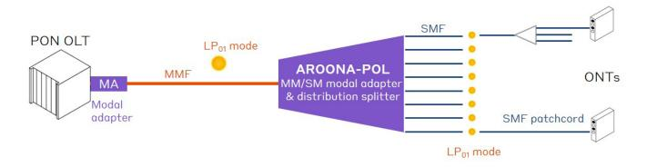
As far as the SM to MM version is concerned, the principle remains the same. Downstream, AROONA-POL splits the SMF signal from OLT and converts it to the  $LP_{o1}$  distribution
